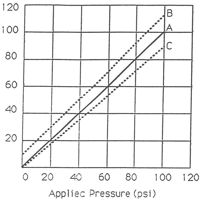
Figure 3-Illustration of Zero Offset, Span Offset, and Sensitivity Error
