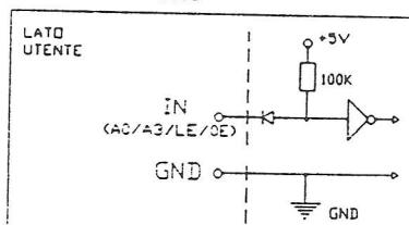
SCHEMA CONNESSIONE USCITE BCD
