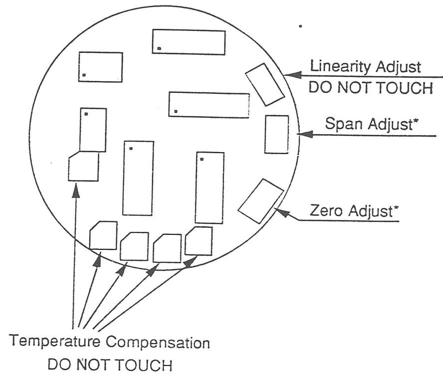
**Figure 2b - Transducer Circuit Layout (typical)**
