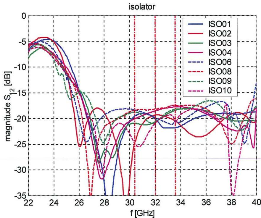
the isolators selected to be mounted in the radiometer are indicated in red
