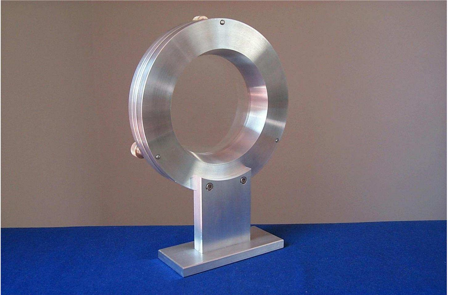
Figure 13: Beam Splitter - front view
