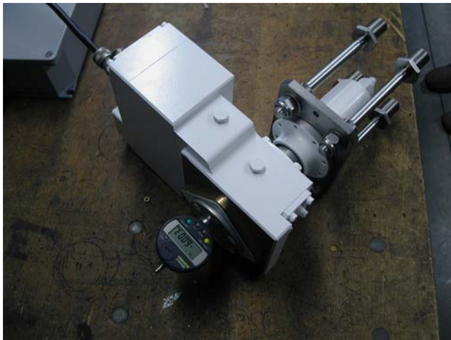
Fig. 3.2 Arrangement of the dial indicator on the moving axis of the actuator
