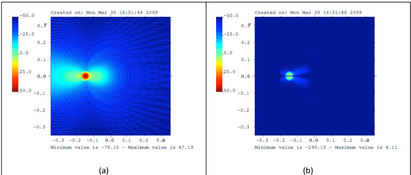
Fig. 11 – Co-polarized and cross-polarized beams with feed shifted 110 mm along x and tilted of 7 deg.
