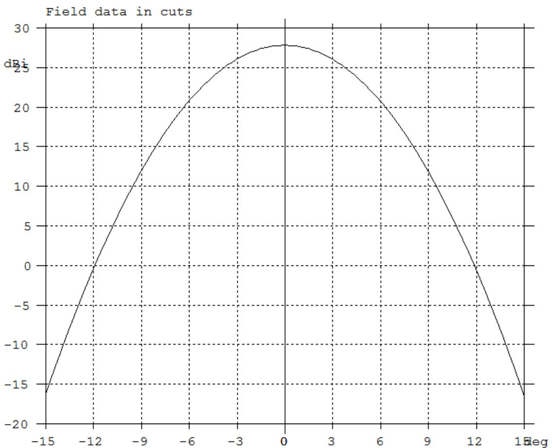
Fig. 5 – Gaussian feed with taper: -12 dB @ 7.8 deg, and -45 dB @ 15 deg.
