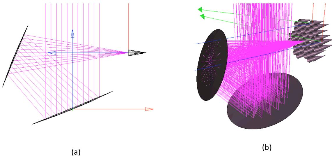
Fig. 4 – (a) Ray tracing of the Dragonian antenna in the xz plane (z-axis in blue); (b) 3D representation of 49 feeds in the FA.
