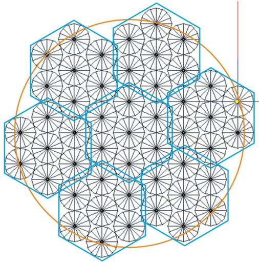
Fig. 1 – Hexagonal arrangement of the feeds in the focal plane. The maximum distance of the outer feeds from the center of the cluster is 108 mm, corresponding to the radius of the external circumference.
