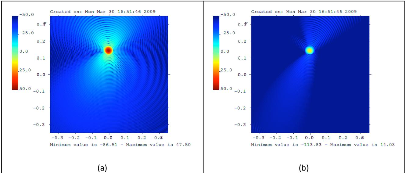
Fig. 16 – Co-polarized and cross-polarized beams with feed shifted -110 mm along y and tilted 8 deg.
