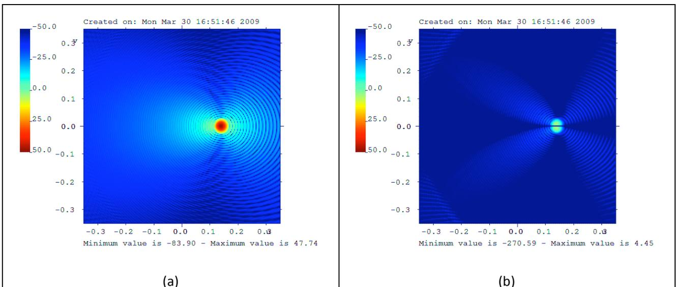
Fig. 12 – Co-polarized and cross-polarized beams with feed shifted -110 mm along x and tilted 7 deg.
