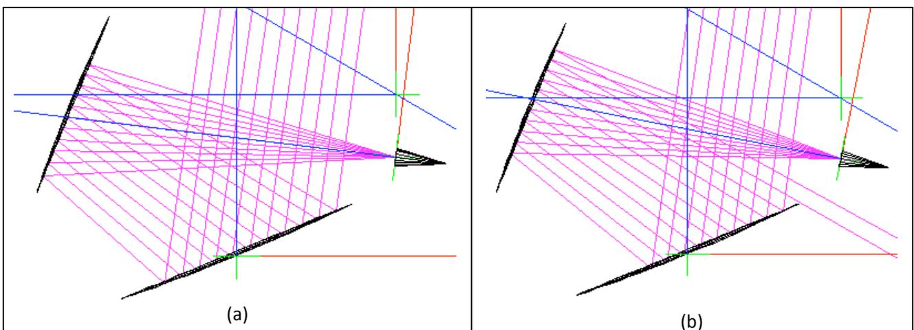
Fig. 8 – Ray tracing in the xz plane for the feed shifted of 110 mm along the negative x-axis and tilt of: (a) 7 deg; (b) 11 deg.
