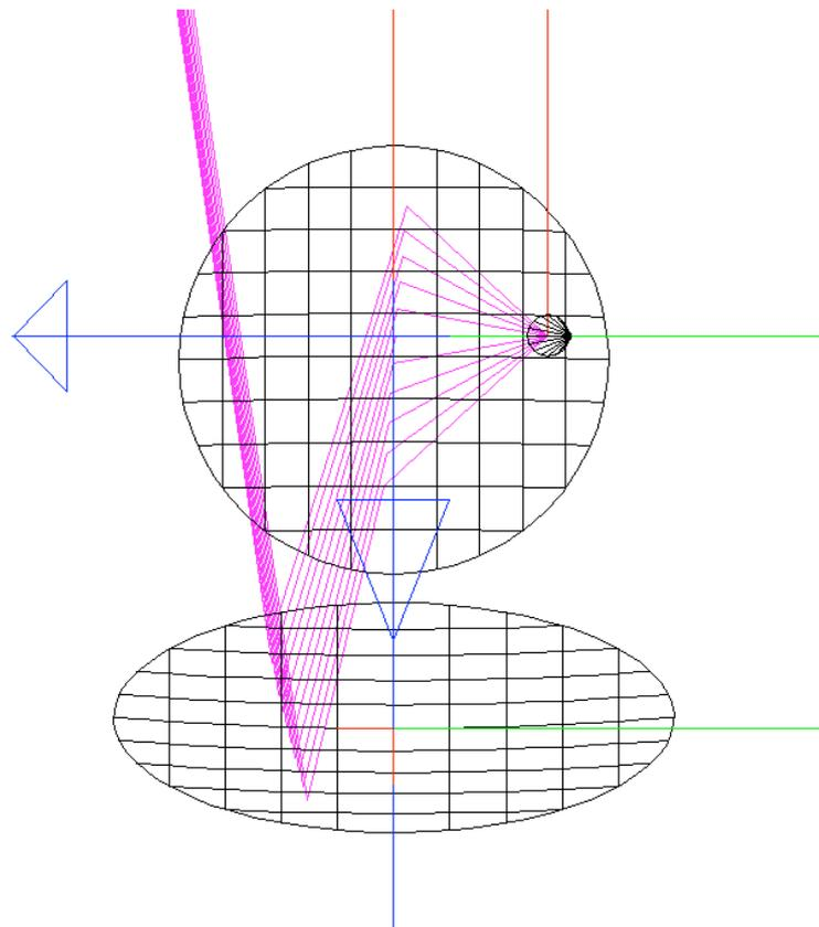
Fig. 13 – Ray tracing in the yz plane for the feed shifted of 110 mm along the positive y-axis and tilt of 11 deg.
