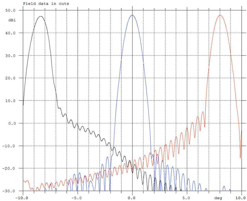
Fig. 9 – Main co-polar antenna beams, in cut  $\phi = 0$  deg, for three different configurations: feed at the center of the FA (blue); feed shifted along x of 110 mm (black); feed shifted along x of -110 mm (red).
