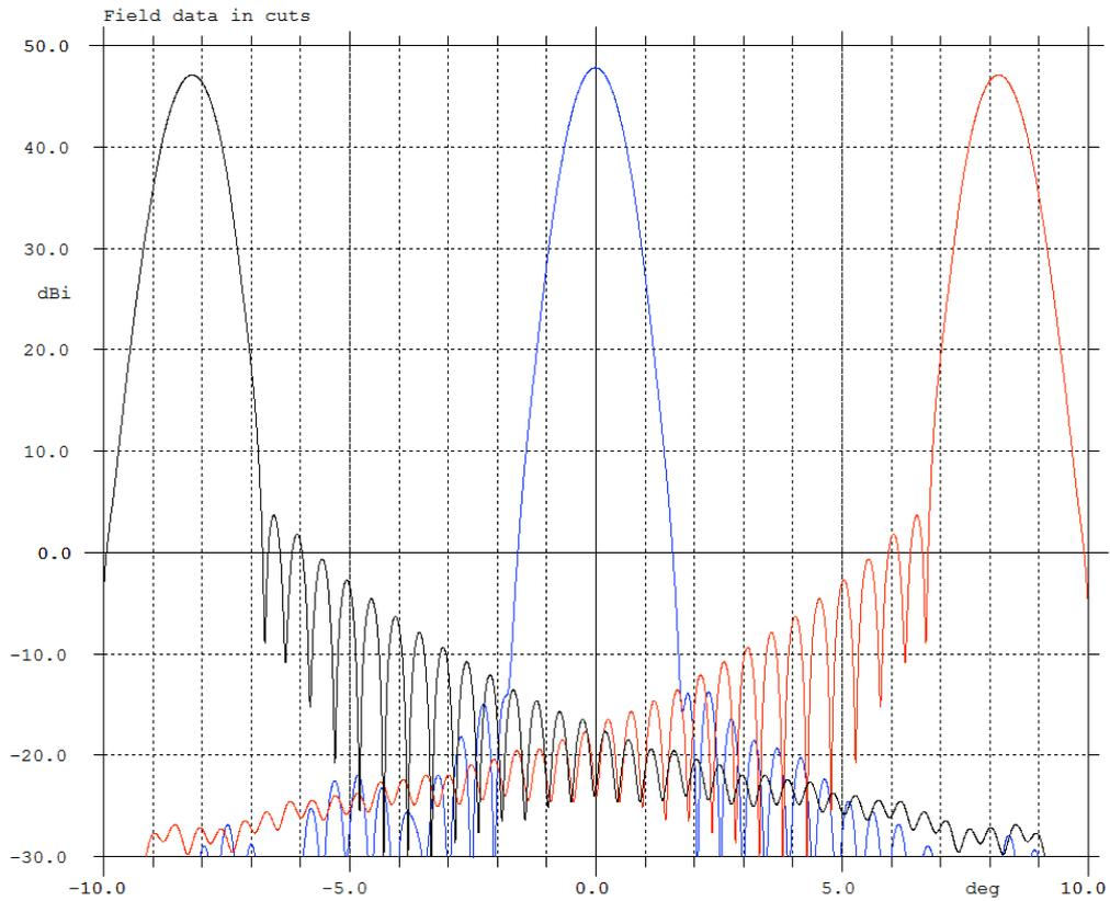
Fig. 14 – Main co-polar antenna beams, in cut  $\phi = 90$  deg, for three different configurations: feed at the center of the FA (blue); feed shifted along  $y$  of 110 mm (black); feed shifted along  $y$  of -110 mm (red).
