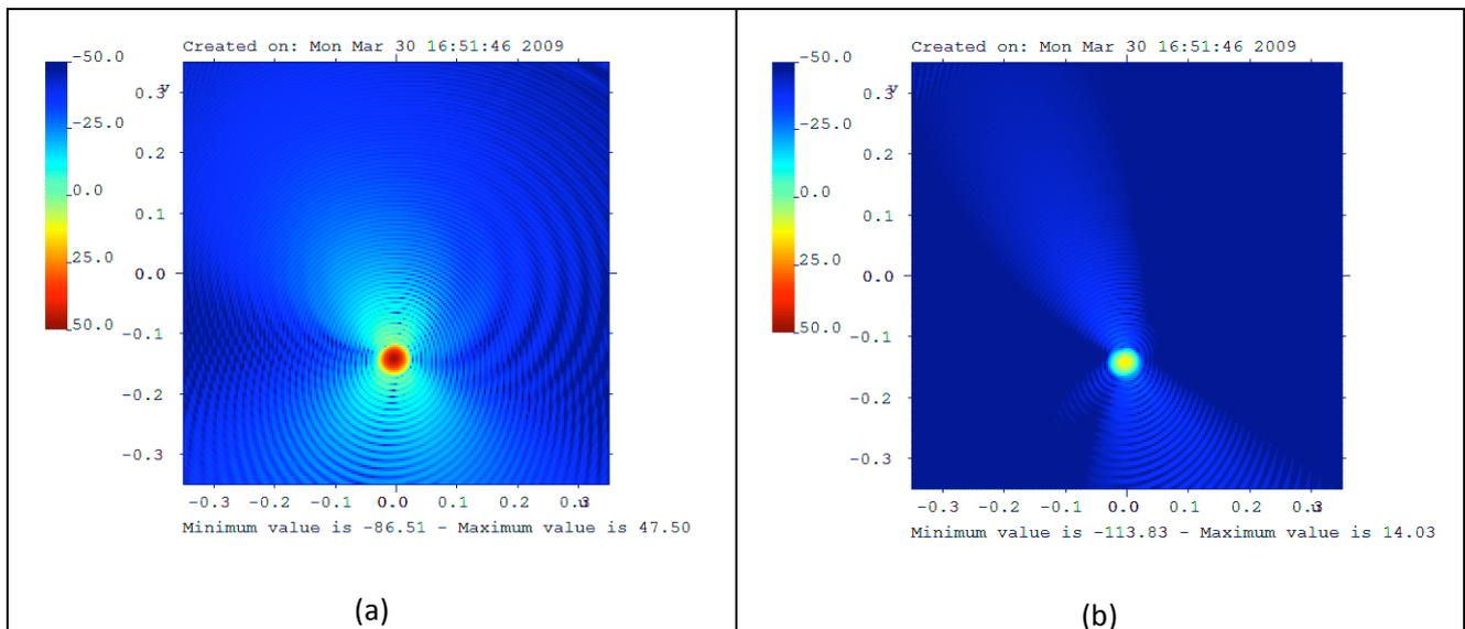
Fig. 15 – Co-polarized and cross-polarized beams with feed shifted 110 mm along  $y$  and tilted 8 deg.
