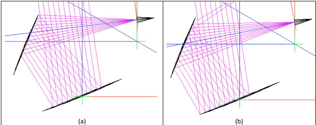
Fig. 7 – Ray tracing in the xz plane for the feed shifted of 110 mm along the positive x-axis and tilt of: (a) 7 deg; (b) 11 deg.
