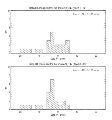
Figure 34: Histogram of the difference between the RA taken from the literature and the ones measured from the Gaussian fit in units of arcsec. Top: Left circular polarization; Bottom: Right circular polarization.
