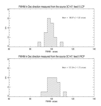
Figure 33: Histogram of the FWHM of the telescope beam (expected  $\approx 100$  arcsec) measured from the Gaussian fit in declination direction. Top: Left circular polarization; Bottom: Right circular polarization.
