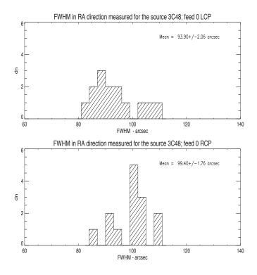
Figure 16: Histogram of the FWHM of the telescope beam (expected  $\approx 100$  arcsec) measured from the Gaussian fit in right ascension direction. Top: Left circular polarization; Bottom: Right circular polarization.
