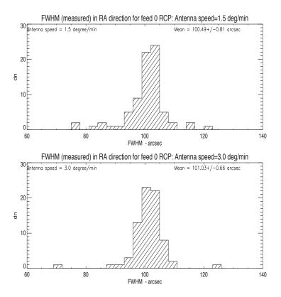
Figure 12: Histogram of the FWHM of the telescope beam ( expected  $\approx 100$  arcsec) measured from the Gaussian fit in right ascension direction for right circular polarization. Top: Scans performed with antenna speed of  $1.5^{\circ}$ /minute; Bottom: Scans performed with antenna speed of  $3.0^{\circ}$ /minute.
