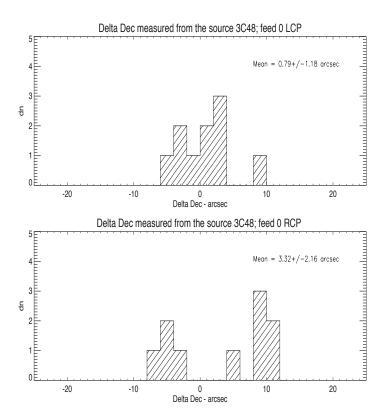
Figure 19: Histogram of the difference between the Dec taken from the literature and the ones measured from the Gaussian fit in units of arcsec. Top: Left circular polarization; Bottom: Right circular polarization.
