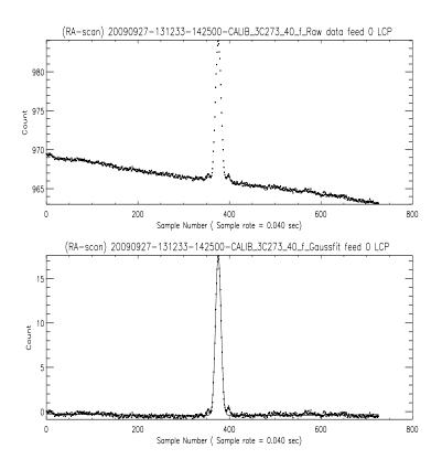
Figure 1: Scan across source 3C273 at an elevation of  $40^{\circ}$  with the central feed for left circular polarization. Top: Raw data, Bottom: Gaussian fit with a  $2^{nd}$  order polynomial background, after baseline subtraction. X-axis represents the sample number (sample rate is 40 ms); Y-axis represents the signal in an arbitrary unit referred as Count.
