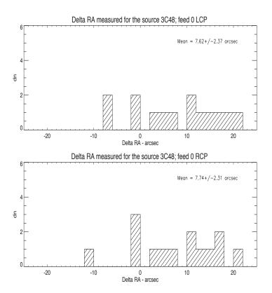
Figure 18: Histogram of the difference between the RA taken from the literature and the ones measured from the Gaussian fit in units of arcsec. Top: Left circular polarization; Bottom: Right circular polarization.
