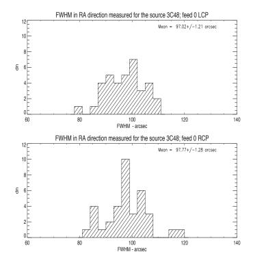
Figure 24: Histogram of the FWHM of the telescope beam ( expected  $\approx 100$  arcsec) measured from the Gaussian fit in right ascension direction. Top: Left circular polarization; Bottom: Right circular polarization.
