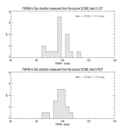
Figure 21: Histogram of the FWHM of the telescope beam (expected  $\approx 100$  arcsec) measured from the Gaussian fit in declination direction. Top: Left circular polarization; Bottom: Right circular polarization.
