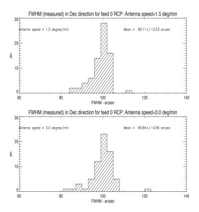
Figure 13: Histogram of the FWHM of the telescope beam (expected  $\approx 100$  arcsec) measured from the Gaussian fit in declination direction for right circular polarization. Top: Scans performed with antenna speed of  $1.5^{\circ}$ /minute; Bottom: Scans performed with antenna speed of  $3.0^{\circ}$ /minute
