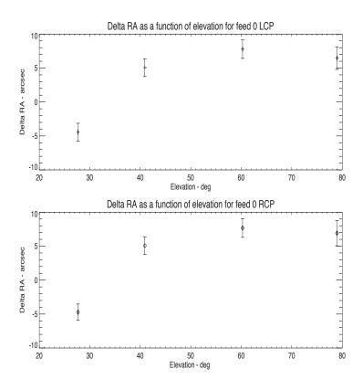
Figure 6: Delta RA (arcsec) versus elevation(degrees). Top: Left circular polarization; Bottom: Right circular polarization
