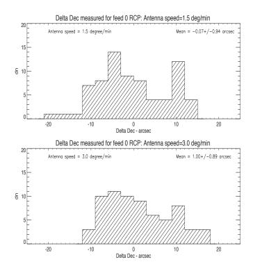
Figure 15: Histogram of the difference between Dec taken from the literature and the ones measured from the Gaussian fit in units of arcsec for right circular polarization. Top: Scans performed with antenna speed of  $1.5^{\circ}$ /minute; Bottom: Scans performed with antenna speed of  $3.0^{\circ}$ /minute
