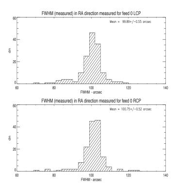
Figure 2: Histogram of the FWHM of the telescope beam (expected  $\approx 100 \text{ arcsec}$ ) measured from the Gaussian fit in right ascension direction. Top: Left circular polarization; Bottom: Right circular polarization.
