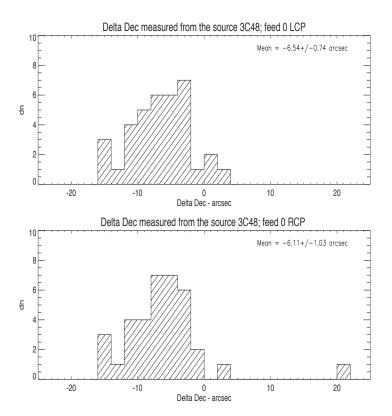
Figure 27: Histogram of the difference between the Dec taken from the literature and the ones measured from the Gaussian fit in units of arcsec. Top: Left circular polarization; Bottom: Right circular polarization.
