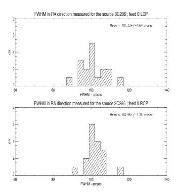
Figure 20: Histogram of the FWHM of the telescope beam ( expected  $\approx 100$  arcsec) measured from the Gaussian fit in right ascension direction. Top: Left circular polarization; Bottom: Right circular polarization.
