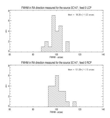
Figure 32: Histogram of the FWHM of the telescope beam ( expected  $\approx 100$  arcsec) measured from the Gaussian fit in right ascension direction. Top: Left circular polarization; Bottom: Right circular polarization.
