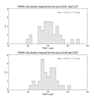
Figure 25: Histogram of the FWHM of the telescope beam (expected  $\approx 100$  arcsec) measured from the Gaussian fit in declination direction. Top: Left circular polarization; Bottom: Right circular polarization.
