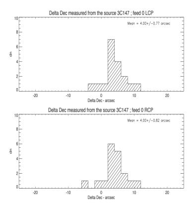
Figure 35: Histogram of the difference between the Dec taken from the literature and the ones measured from the Gaussian fit in units of arcsec. Top: Left circular polarization; Bottom: Right circular polarization.
