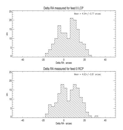
Figure 4: Histogram of the difference between the RA taken from the literature and the ones measured from the Gaussian fit in units of arcsec. Top: Left circular polarization; Bottom: Right circular polarization.
