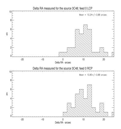
Figure 26: Histogram of the difference between the RA taken from the literature and the ones measured from the Gaussian fit in units of arcsec. Top: Left circular polarization; Bottom: Right circular polarization.
