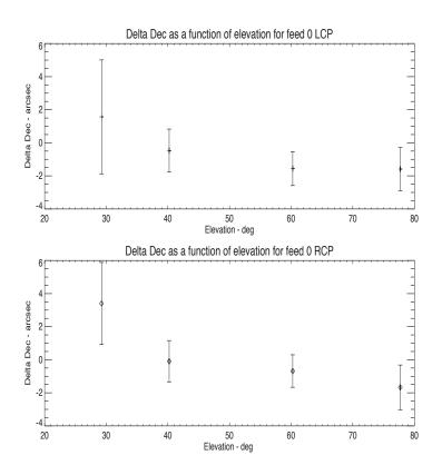
Figure 7: Delta Dec (arcsec) dependence on the elevation (degrees). Top: Left circular polarization; Bottom: Right circular polarization
