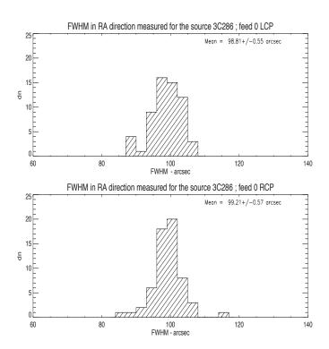
Figure 28: Histogram of the FWHM of the telescope beam (expected  $\approx 100$  arcsec) measured from the Gaussian fit in right ascension direction. Top: Left circular polarization; Bottom: Right circular polarization.
