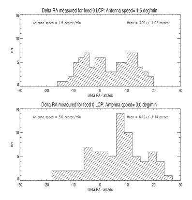
Figure 10: Histogram of the difference between RA taken from the literature and the ones measured from the Gaussian fit in units of arcsec for left circular polarization. Top: Scans performed with antenna speed of  $1.5^{\circ}$ /minute; Bottom: Scans performed with antenna speed of  $3.0^{\circ}$ /minute
