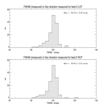
Figure 3: Histogram of the FWHM of the telescope beam (expected  $\approx 100$  arcsec) measured from the Gaussian fit in declination direction. Top: Left circular polarization; Bottom: Right circular polarization.
