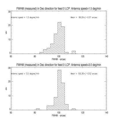
Figure 9: Histogram of the FWHM of the telescope beam (expected  $\approx 100$  arcsec) measured from the Gaussian fit in declination direction for left circular polarization. Top: Scans performed with antenna speed of  $1.5^{\circ}$ /minute; Bottom: Scans performed with antenna speed of  $3.0^{\circ}$ /minute
