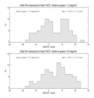
Figure 14: Histogram of the difference between RA taken from the literature and the ones measured from the Gaussian fit in units of arcsec for right circular polarization. Top: Scans performed with antenna speed of  $1.5^{\circ}$ /minute; Bottom: Scans performed with antenna speed of  $3.0^{\circ}$ /minute
