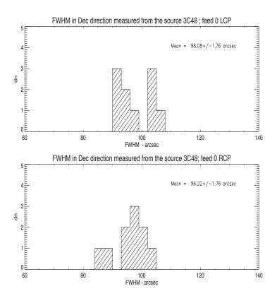
Figure 17: Histogram of the FWHM of the telescope beam (expected  $\approx 100$  arcsec) measured from the Gaussian fit in declination direction. Top: Left circular polarization; Bottom: Right circular polarization.
