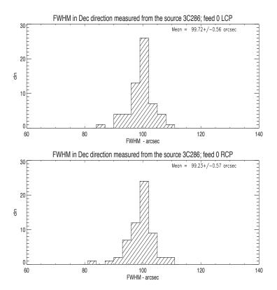
Figure 29: Histogram of the FWHM of the telescope beam (expected  $\approx 100$  arcsec) measured from the Gaussian fit in declination direction. Top: Left circular polarization; Bottom: Right circular polarization.
