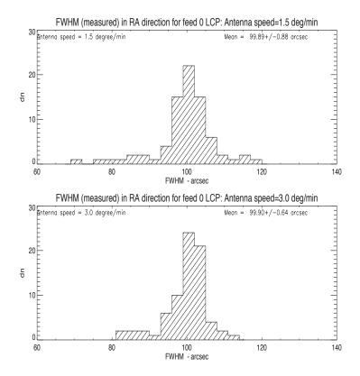
Figure 8: Histogram of the FWHM of the telescope beam (expected  $\approx 100$  arcsec) measured from the Gaussian fit in right ascension direction for left circular polarization. Top: Scans performed with antenna speed of  $1.5^{\circ}$ /minute; Bottom: Scans performed with antenna speed of  $3.0^{\circ}$ /minute.
