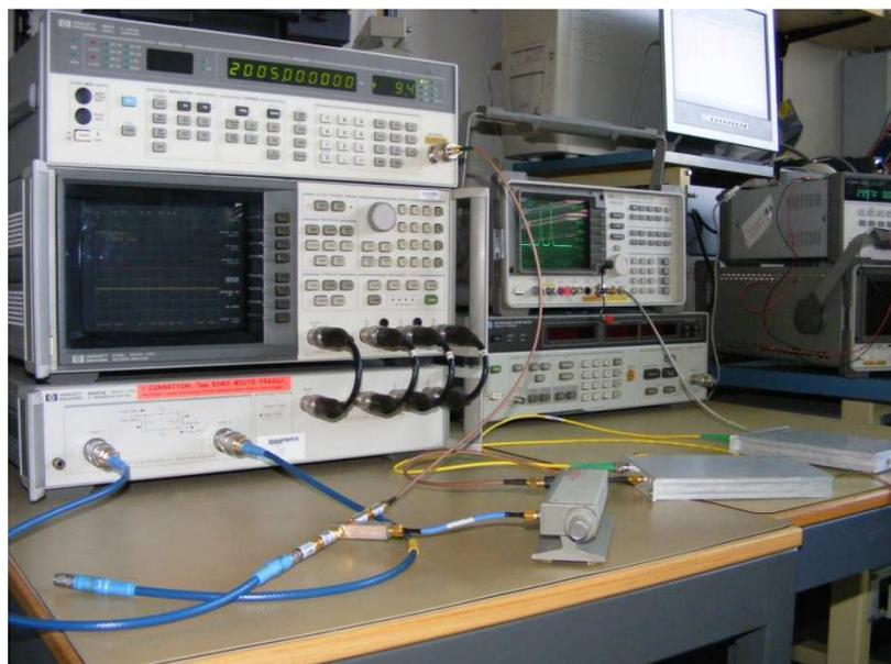
Figure 13 – IP3 measurement set up.
