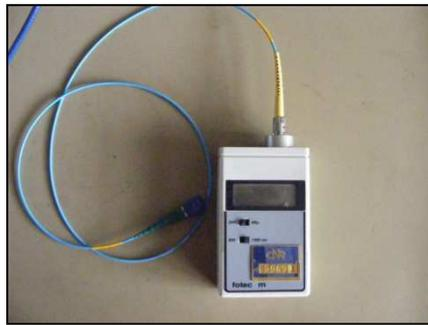
Figure 3 – Optical power meter.
