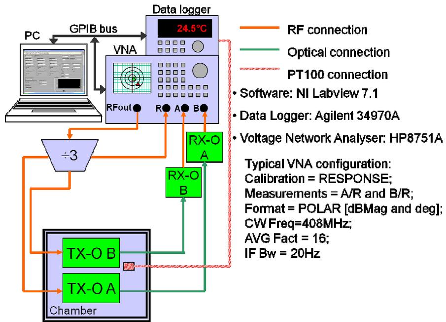
Figure 27 – Ripple measurement block diagram set up.
