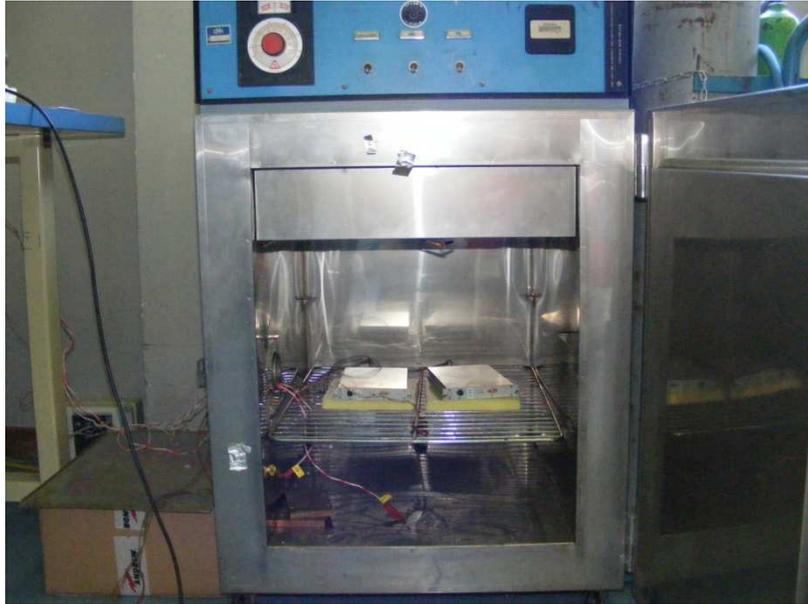
**Figure 29** – Optical TXs inside the chamber.
