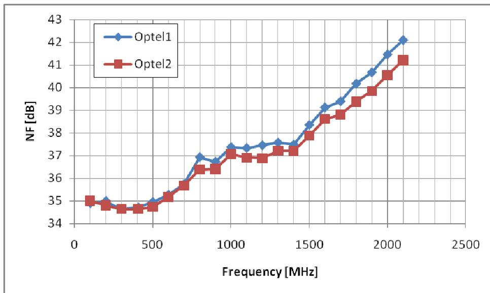
Figure 19 – Optel1 and Optel2 NF link measurements (with HP8564E).
