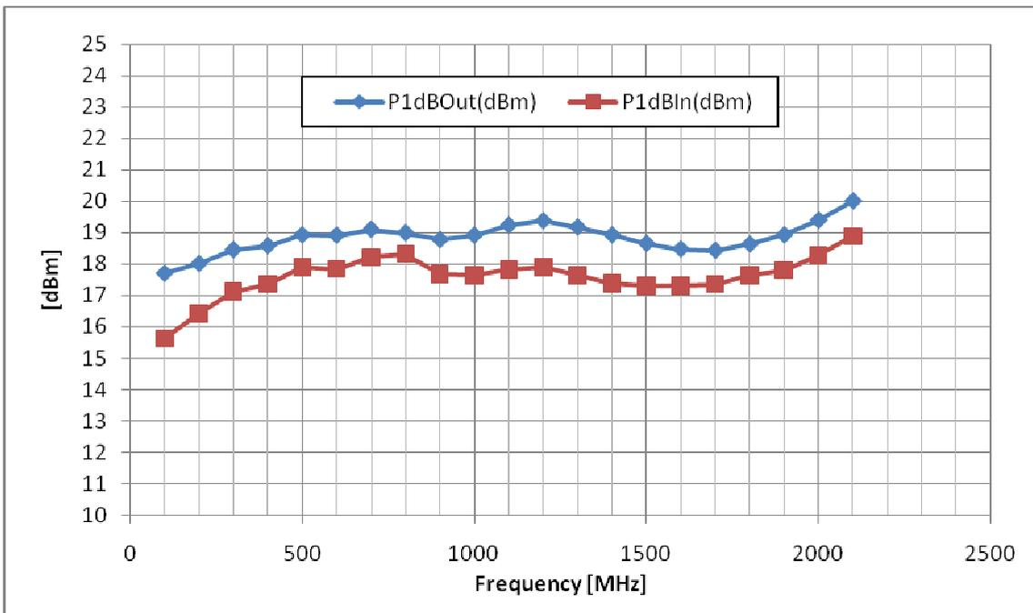
Figure 24 – Optel1 Input and Output 1dB compression point.
