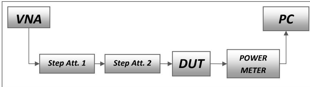
Figure 21 – P1dB measurement set up block diagram.
