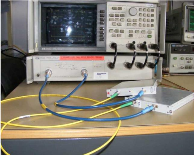
Figure 4 – S-parameters measurement set up.
