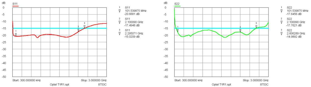
Figure 10 – Optel1 input (left) and output (right) matching (horizontal sky blue line = IRA goal specification).
