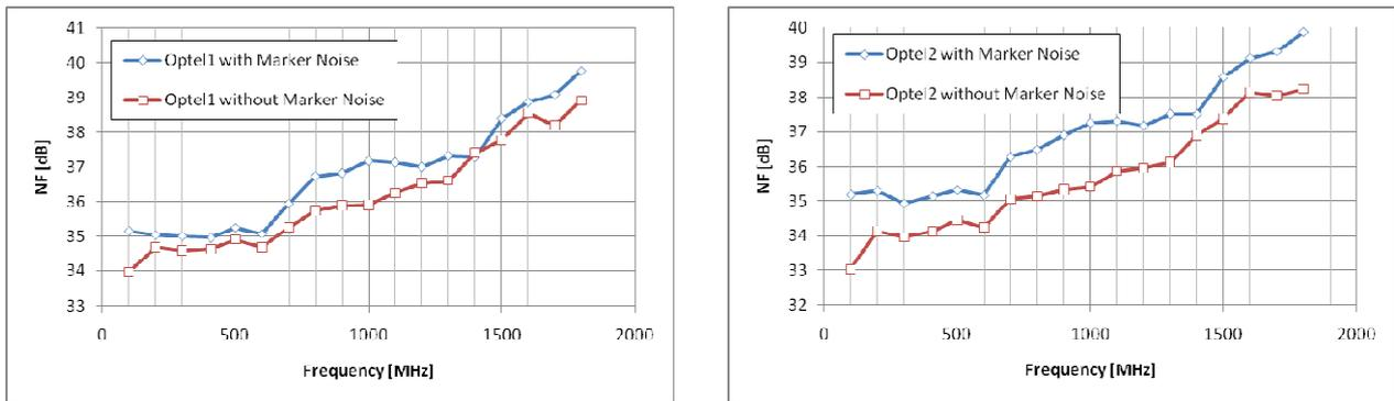
Figure 20 – NF measurements comparison: with and without Marker Noise.
