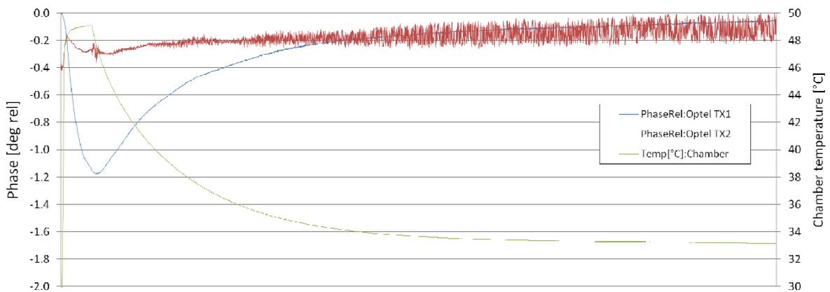
Figure 31 – Optel TX1 and TX2 phase variation vs temperature (horizontal axes is time, not showed).
