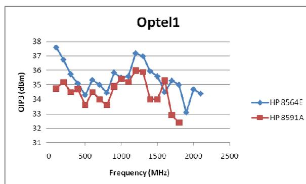
Figure 16 – OIP3 link measurements: comparison between the spectrum analysers.
