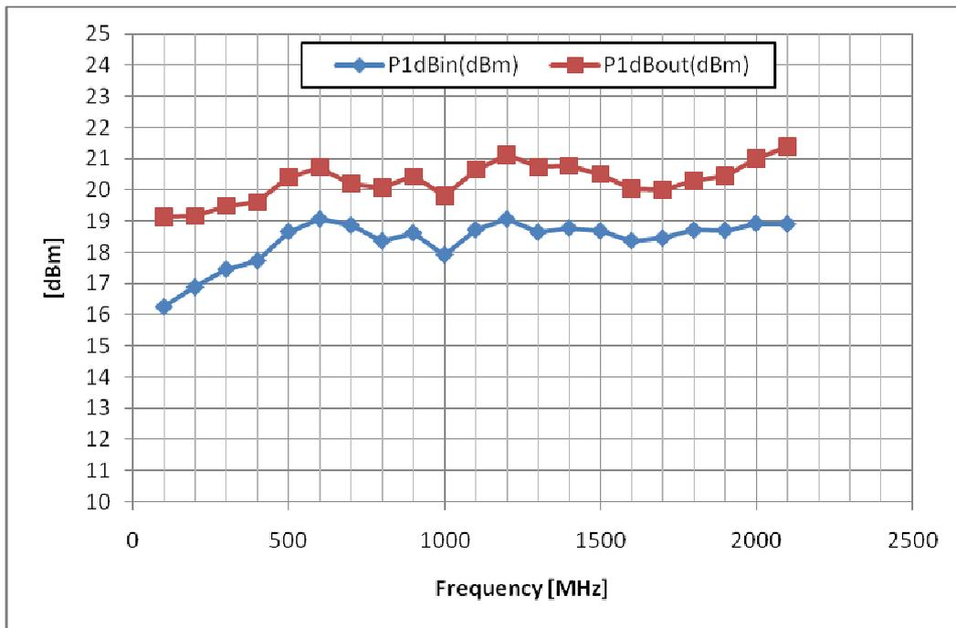
Figure 25 – Optel2 Input and Output 1dB compression point.
