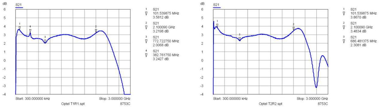
Figure 6 - Gain (S21): Optel1 (left) and Optel2 (right).
