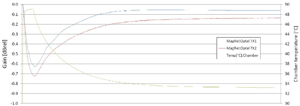
Figure 30 – Optel TX1 and TX2 gain variation vs temperature (horizontal axes is time, not showed).
