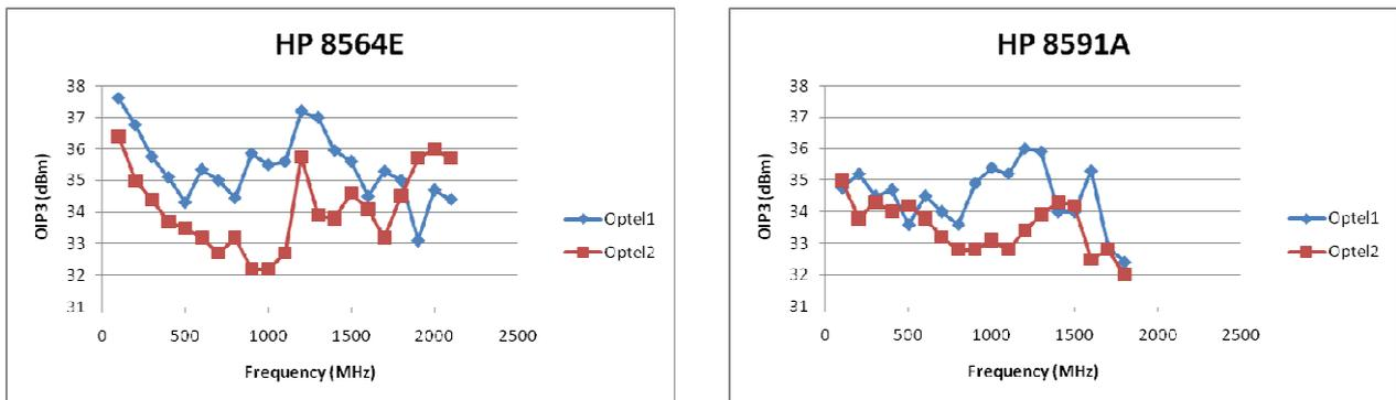
Figure 15 – OIP3 link measurements with HP 8564E (left) and HP 8591A (right) spectrum analysers.
