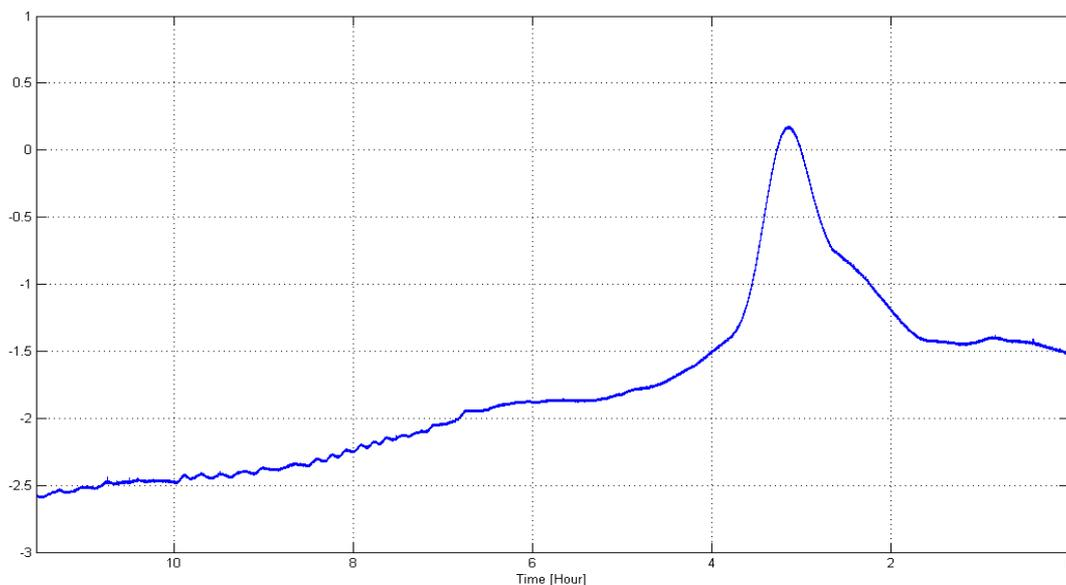
Figure 26 – Total power ripple on a detected transit of Cas-A with a single BEST-1 RX.
