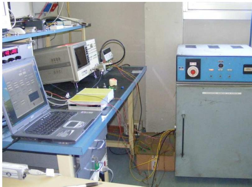
Figure 28 – Ripple measurement set up.
