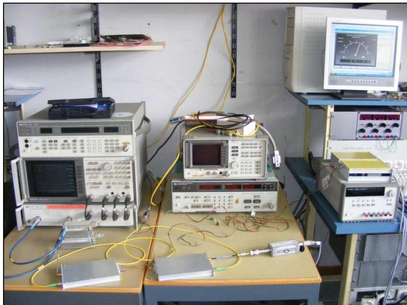
Figure 22 – P1dB measurement set up.
