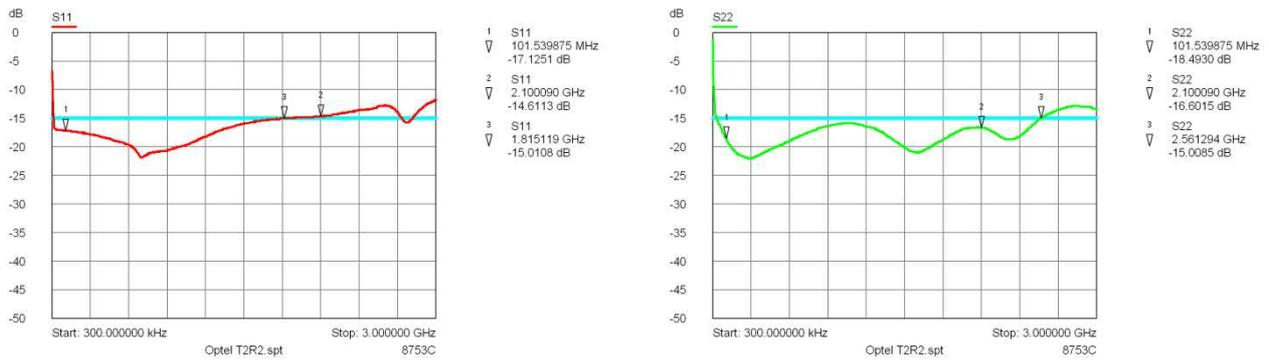
Figure 11 – Optel2 input (left) and output (right) matching (horizontal sky blue line = IRA goal specification).
