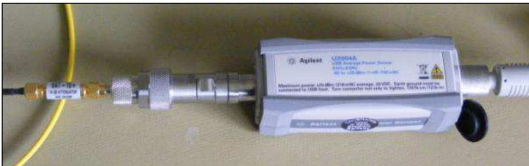
Figure 23 – Agilent Power Meter with 10dB attenuator.
