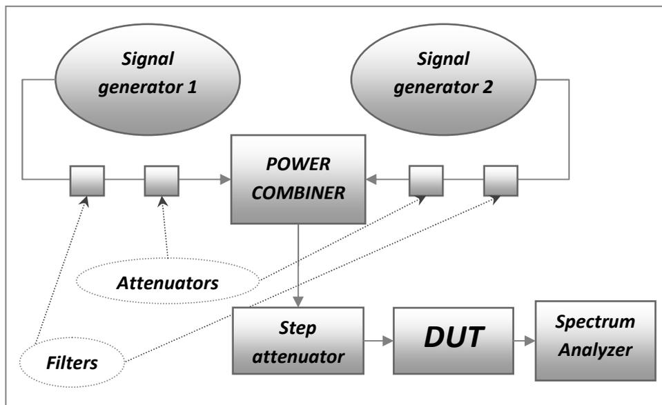
Figure 12 – IP3 measurement set up block diagram.
