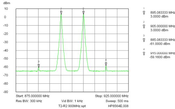
Figure 14 – Fundamentals tones and their relative third order intermodulation products.
