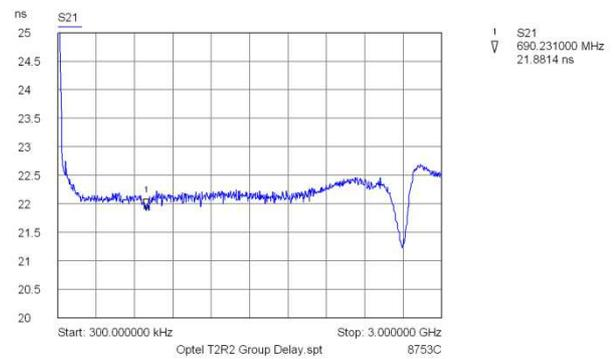
Figure 9 – Optical link group delay: Optel 1 (left) and Optel 2 (right).
