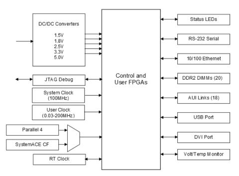
Fig. 6: Block diagram of the BEE2 board general architecture
