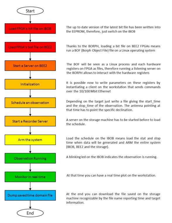
Fig. 27: State Machine Flow Chart
