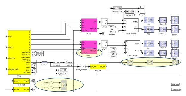
Fig. 21: Propagating the sync signal with intermediate block latencies
