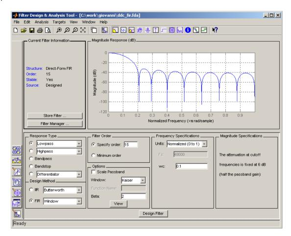
Fig. 17: design parameters of the FIR filter inside the DDC block.
