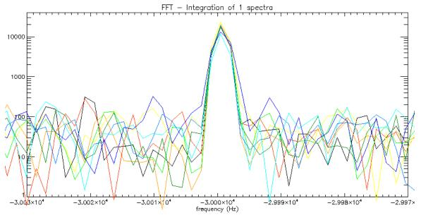
Fig. 36: Frequency 407.970kHz sampled using the Rohde&Schwarz SMX as clock sampler. The read frequency results exactly 407.970kHz
