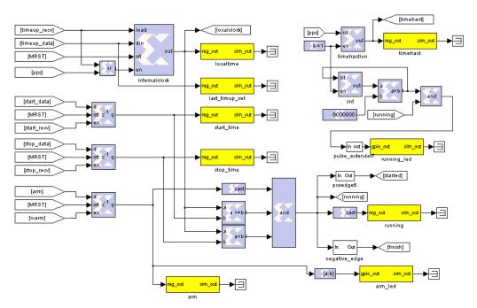
Fig. 20: IBOB Timing registers
