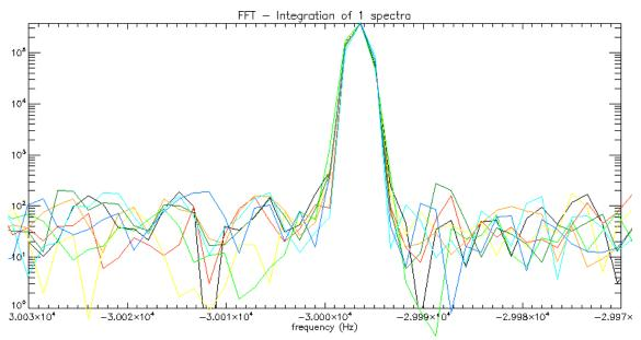
Fig. 35: Frequency 407.970kHz sampled using the HP 8657B as clock sampler. The read frequency results 407.974kHz, 4Hz difference
