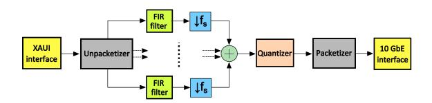
Fig. 24: BEE2 firmware architecture
