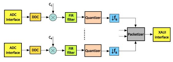
Fig. 15: IBOB firmware architecture
