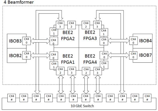
Fig. 11: 4 Parallel Beamformer System Connection Scheme (control and storage must be connected as in the previous scheme)
