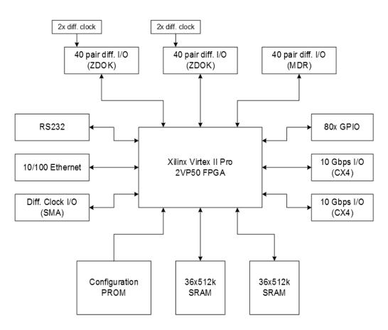
Fig. 2: Block diagram of the Ibob board general architecture
