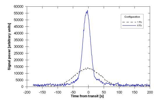
Fig. 40: Transit of Virgo-A observed by a single E-W receiver (dashed black line) and by a synthetized beam of 4 receivers (continuous blue line).
