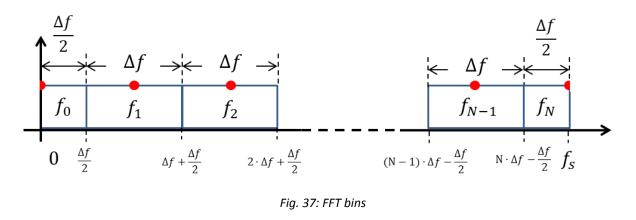
The above picture shows how the red points (FFT lines) are the center of the FFT bins (or FFT channels) of  $\Delta f$  width (unless the first and the last channel that have half width) bounded within
