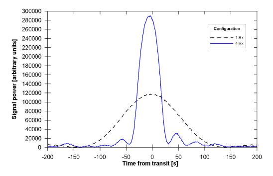
Fig. 39: Transit of Cygnus-A observed by a single E-W receiver (dashed black line) and by a synthetized beam of 4 receivers (continuous blue line).
