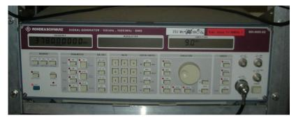
Fig. 12: Picture of the Local Oscillator set to 378MHz in input to the MIXER to generate a IF of 30MHz
