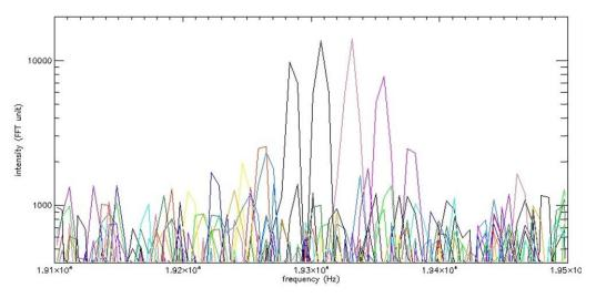
Fig. 29: The doppler shift of the debris ID 18096. Animating this plot the peak moves from right to left
