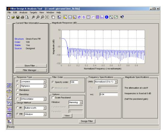
Fig. 25: Design parameters of the FIR filter synthesized in the bee2.
