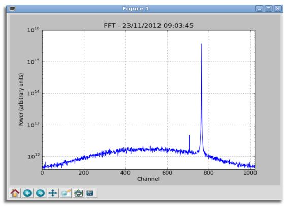
Fig. 28: A real time FFT plot observing a debris in a bistatic radar configuration
