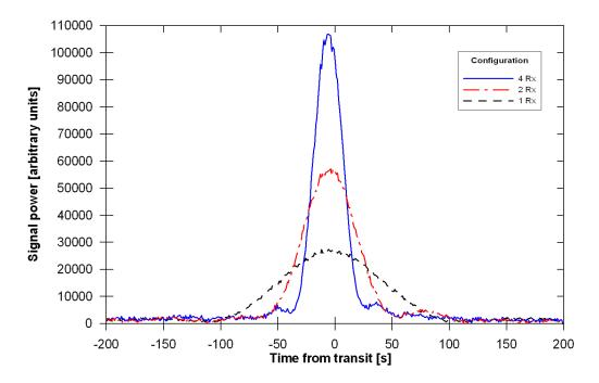
Fig. 41: Transit of Taurus-A observed by a single E-W receiver (dashed black line), by a synthetized beam of 2 receivers (dashed dotted red line) and of 4 receivers (continuous blue line)
