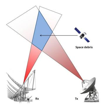
Fig. 1: Bistatic radar configuration geometry.
