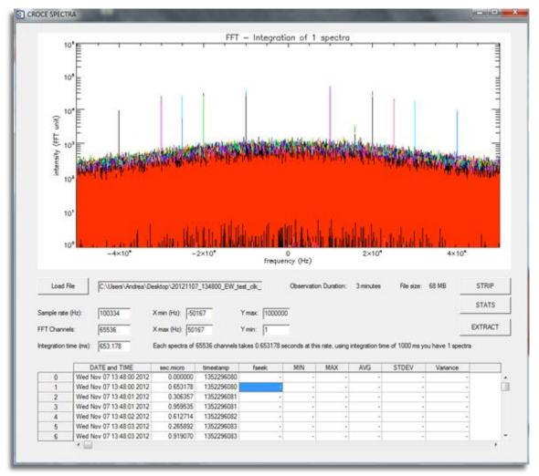
*Fig. 34: Overplotting FFTs of the entire file you can recognize the frequencies used for the test.*
