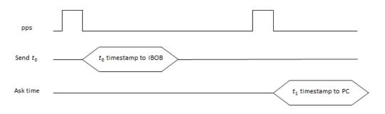
Fig. 19: Time diagram of the time update procedure
