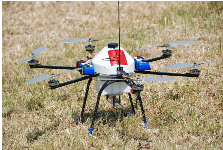
Fig. 9 - Hexacopter equipped with RF transmitter and telescopic dipole.
