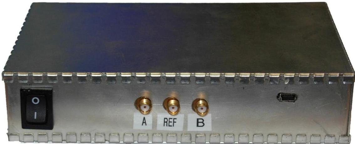
A second unit has been realized. It is a USB pocket synthesizer which needs only of a 220VAC-5VDC switching power supply (Traco Power TMLM 10105, Input 100-240VAC, 50-60Hz, Output 5VDC / 2000mA).
