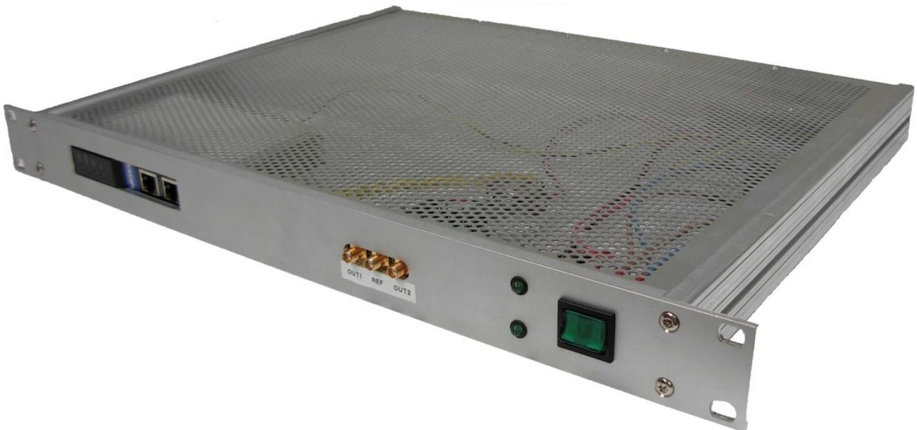
The front panel provides a button switch to power on and off the module, two green LEDs indicating if 5 Volts modules are powered, the SMA connectors for RF input/output of the clock synthesizer and the Ethernet port of the TCP/RS-232 converter. On the rear panel you will find the 220V socket with the fuse.
