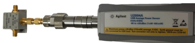
Figure 13: USB power sensor (Agilent U2004A) connected to a directional coupler for the measurement of the signal power level.
