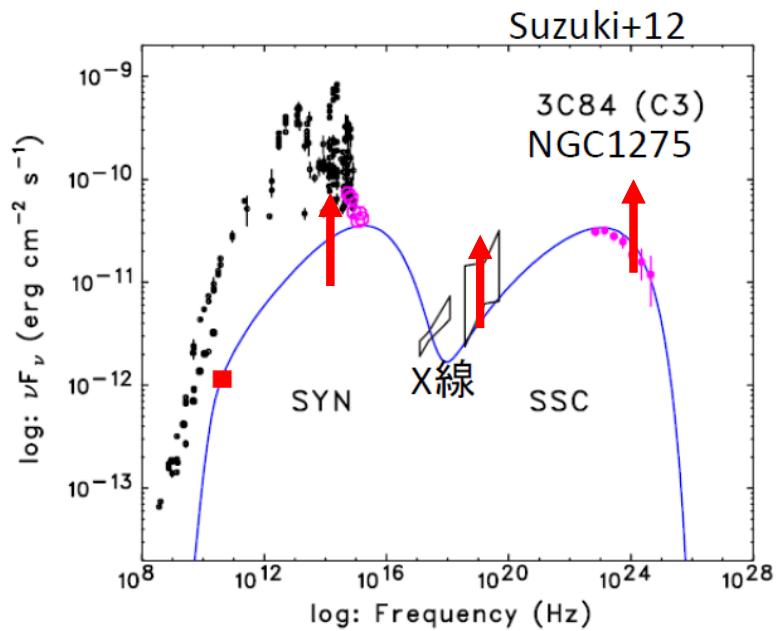
The flux of NGC1275 has been increasing from radio, optical/UV, X-ray, and GeV gamma-ray, without any large change of SED shape.
