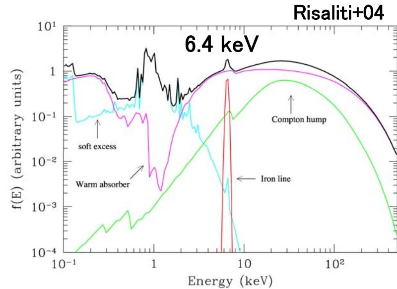
Precise line spectroscopy with X-ray calorimeter is promising to measure a Fe-K line profile (center energy, width and shape, line structure ...)
