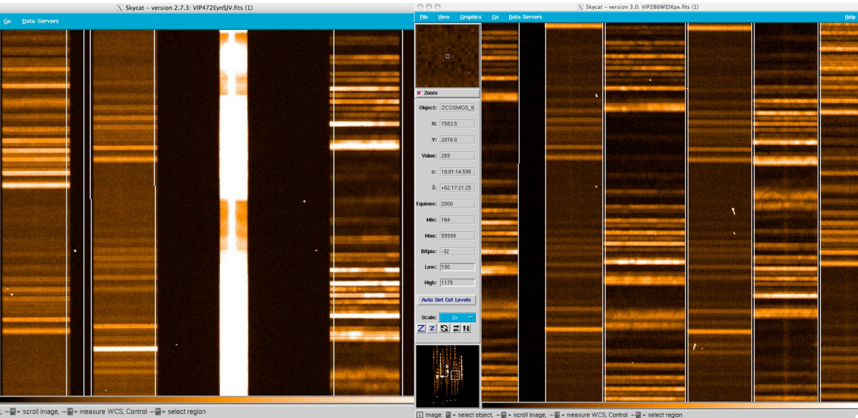
Many fake detections are expected at slit edges in case of bad spectra location
