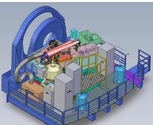
SPHERE: Spectro-Polarimetric High-contrast Exoplanet REsearch. IR imager and spectrograph, NIR Integral Field Spectrograph, visible polarimeter (Goal: at Telescope in winter 2010)
