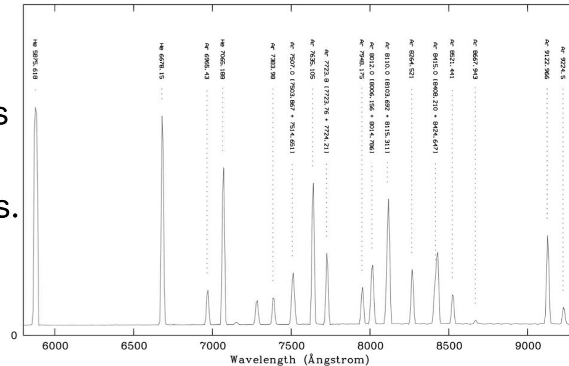
One or more arc exposures are used to build the msLamp.
