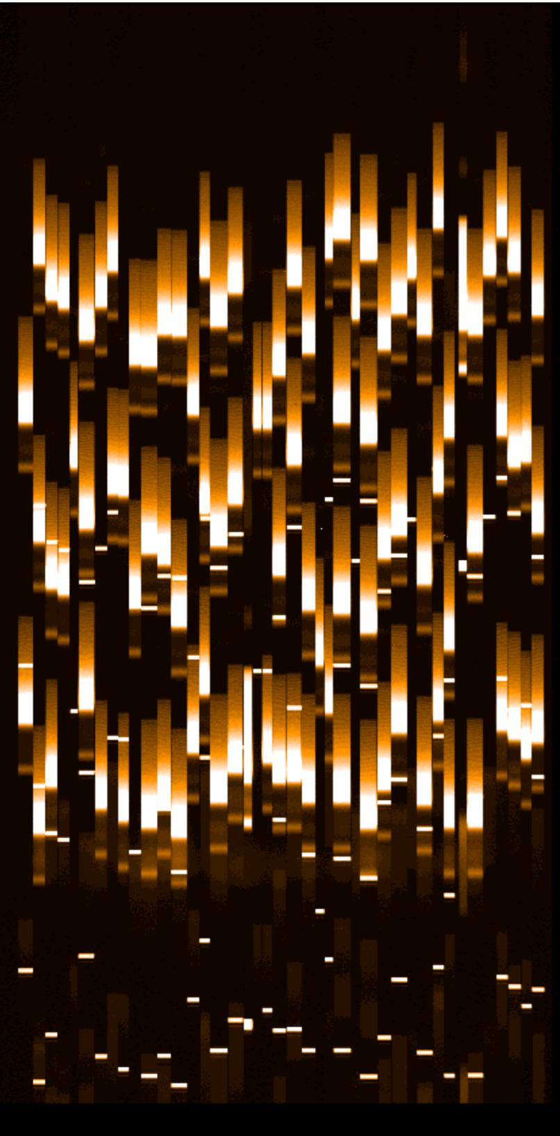
Flat-field: is the efficiency map of the CCD, since the response of each pixel can vary. In imaging it is obtained with a uniform illumination of the CCD (sky or dome flat); each raw image must be bias subtracted and flat-field normalized.
