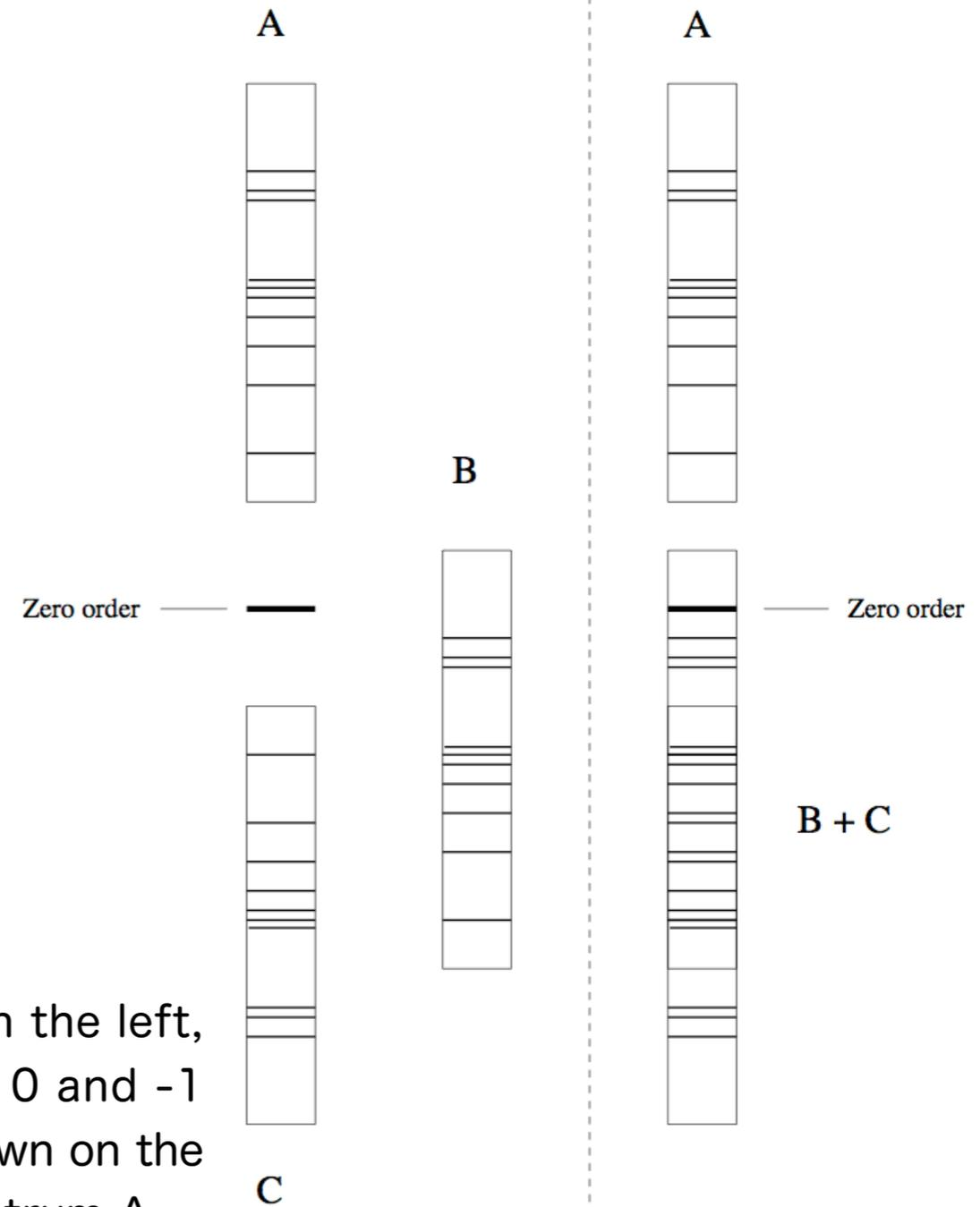
Contamination from orders 0 and -1 in multiplexed spectra. On the left, the first order spectra A and B are shown, together with the 0 and -1 orders of spectrum A. If spectra A and B are multiplexed, as shown on the right, spectrum B is contaminated by the 0 and -1 orders of spectrum A.
