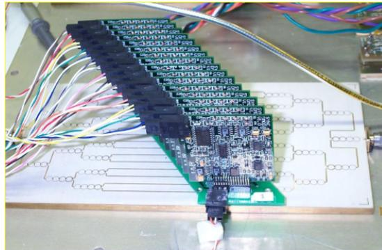
2004-2008: Wide-band analogue correlator on ATCA, 2.4 arcmin FoV, fast scanning at 15 deg/min, 54ms sampling.
