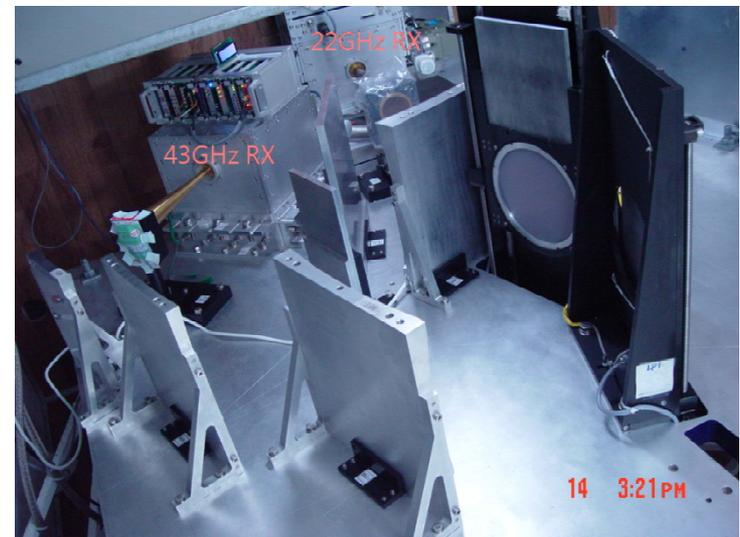
KVN Multi-Frequency Receiver installed at Yonsei antenna receiver room
