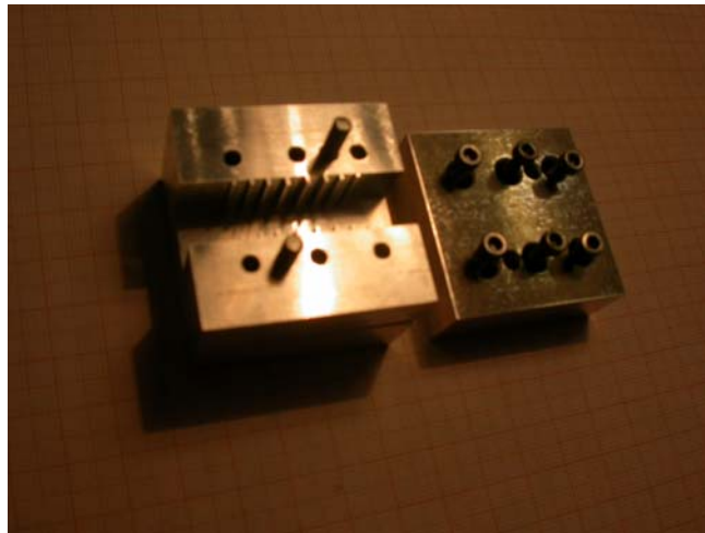
Fig. 3: Differential phase shifter prototype
