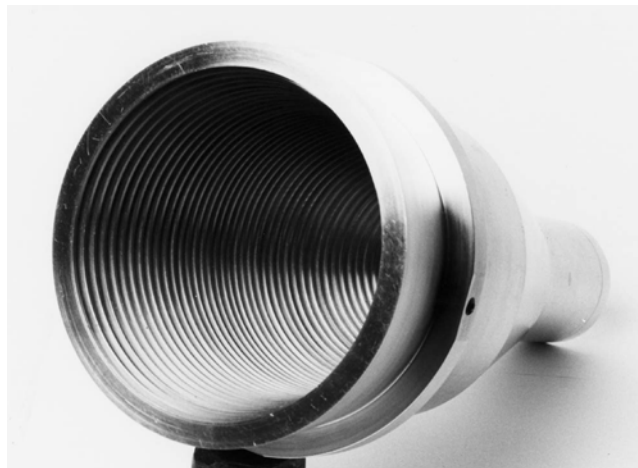
Fig. 2.1.7 . Photo of the corrugated horn for the array receiver.
