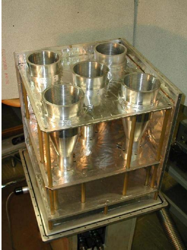
Fig. 2.3.2 Feed horns installed into the dewar.
